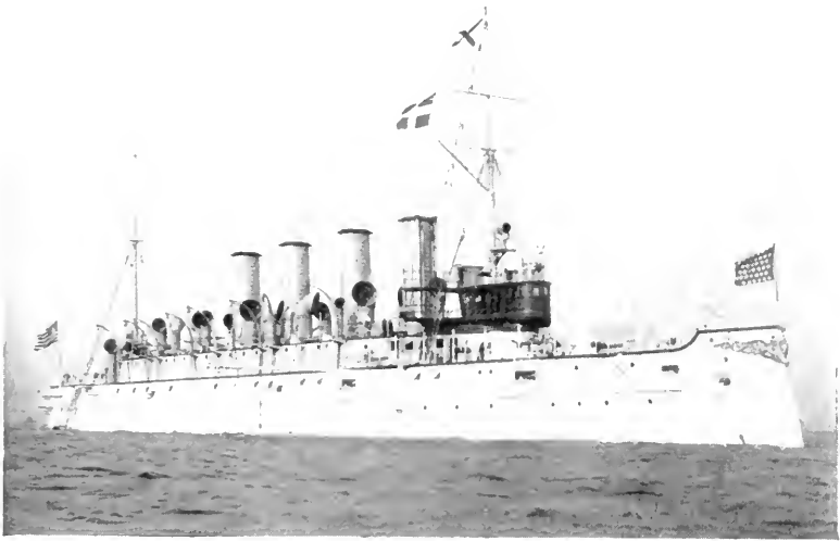
U. S. BATTLE SHIP COLUMBIA, 7744 TONS DISPLACEMENT. Length 412 ft., beam 38, draft 24. Built by Wm. Cramp & Sons, Phila., Pa. Copyright 1895, by J. S. Johnston, N. Y.
